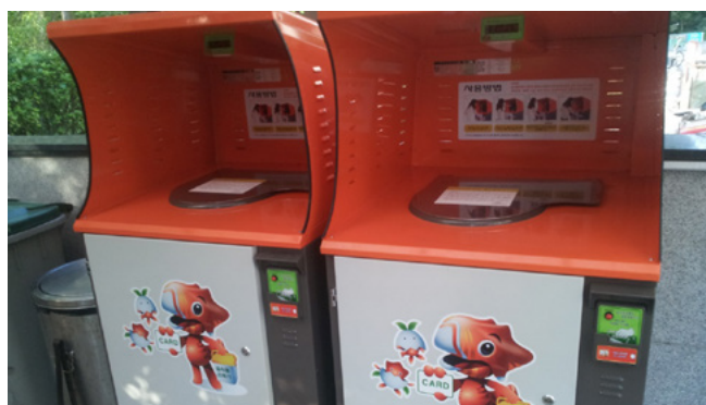
Enabling pay-as-you-throw food-waste recycling using smart scales and radio frequency identification (RFID) technology. Photo credit: Wikimedia
